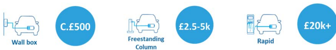
Figure 3. Typical installation costs (excluding chargers).
